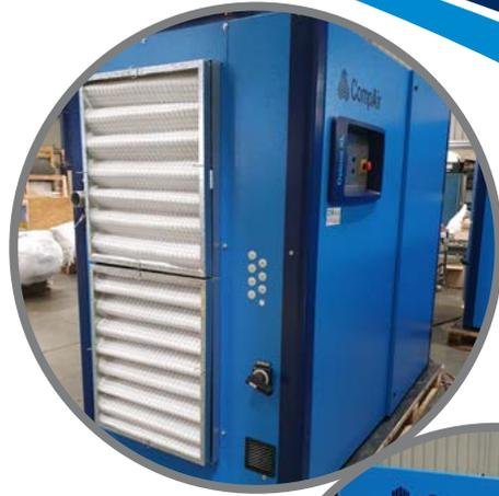
CompAir's F Series dryers provide high quality heat exchange with minimal pressure loss, and a +3°C pressure dewpoint. Simple to operate and maintain, with a compact, space saving design and patented heat exchanger technology, F Series dryers are engineered to help operators to significantly reduce operating costs.
