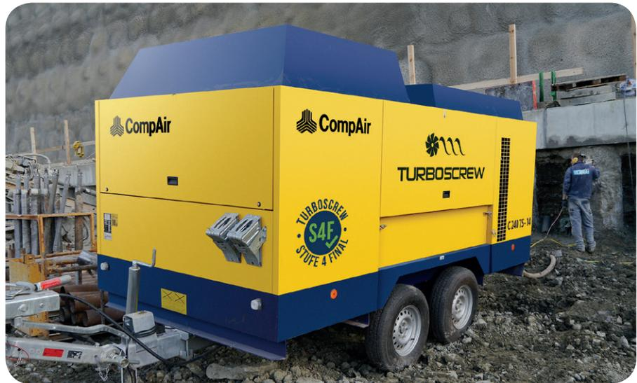
**The new bi-turbo machine at Max Bögl has 14 bar operating pressure and already meets the rigorous requirements of the EU 4 Emissions Standard.**
