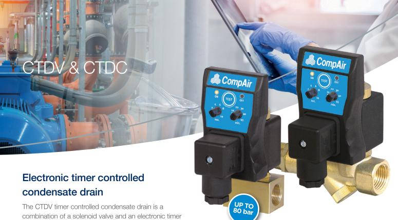
designed to automatically remove condensate from compressed air systems. The CTDC in addition, has an integral ball valve and a strainer, all in the same body.
