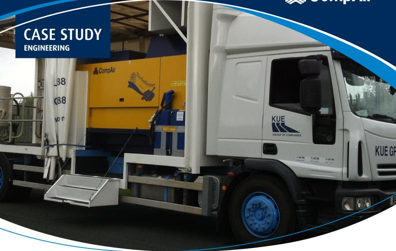
Using patented bi-turbo technology, the TurboScrew compressors are engineered with two turbochargers powering a CompAir screw compressor unit, with the addition of an engine exhaust gas turbine to pre-compress the inlet air before it enters the compression chamber.
