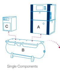
By mounting the components on the receiver, the **foot print** required is reduced by up to 55%.
