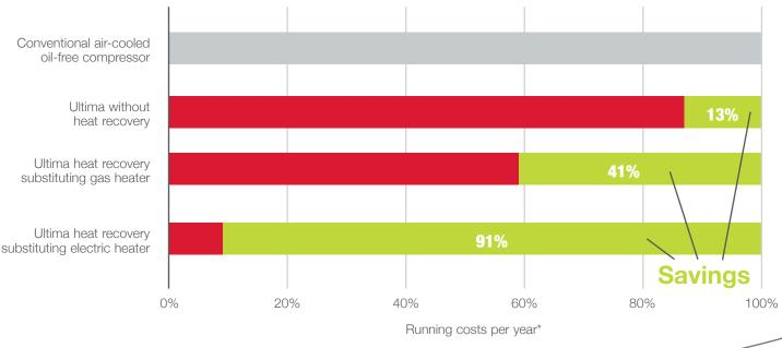
\*Operation @ 20m³/min 8 bar, 4.000 hours per year, electricity price 15 ct/kWh, gas price 5 ct/kWh
