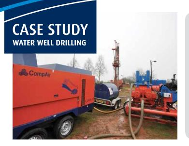
thorough research into the portable compressor market, we chose to purchase a new 17 bar (250 psi), C230TS-17 TurboScrew compressor from CompAir. Our key buying points were; improved fuel efficiency, savings in plant transport, improved health and safety through manoeuvrability, and, very importantly, confidence in the brand. CompAir ticked all of the boxes."
