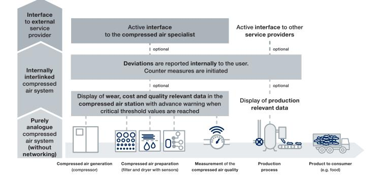
Fig. 2: Possibilities of networking using the example of a compressed air system
